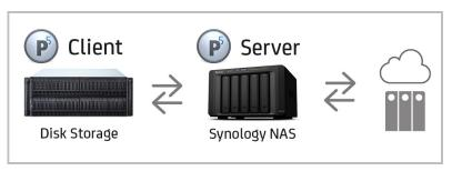
Archiware P5 runs on Synology NAS devices with the DSM operating system 5.2+ and an Intel x86 64-Bit processor.
