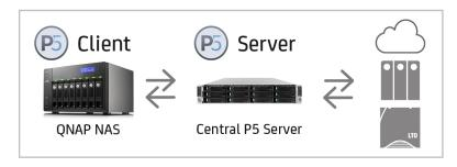
Archiware P5 can be combined with a QNAP NAS using two different setups. In the first setup, P5 acts as a central server, which synchronizes, backs up and clones data from the QNAP NAS onto the desired target (disk, tape or cloud). The QNAP NAS is connected to the central P5 server as direct attached storage or as a P5 client
