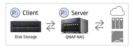
Additionally, the Storage and Snapshots Manager in QTS 4.3 allows QNAP NAS devices to be used as a repository for Backup2Go. This enables mobile backups of laptops and desktops on central disk storage at very low cost per unit and with minimal administration.
