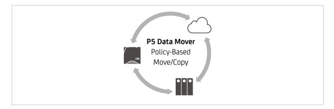
The **P5 Data Mover** is an extension of the P5 Archive module. It offers policybased moving and copying of archived data between tape, cloud and disk storage. This HSM-like extension offers flexibility for any storage strategy. Data can easily be migrated or copied between storage tiers:
