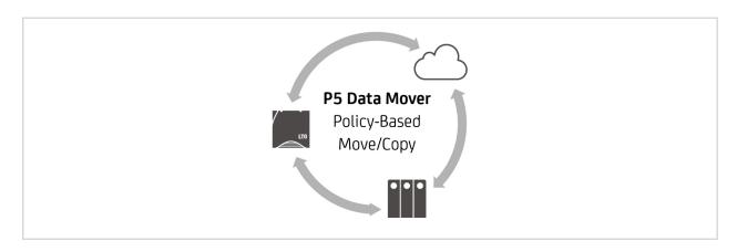
The **P5 Data Mover** is an extension of the P5 Archive module. It offers policy-based moving and copying of archived data between tape, cloud and disk storage. This HSM-like extension offers flexibility for any storage strategy. Data can easily be migrated or copied between storage tiers:
